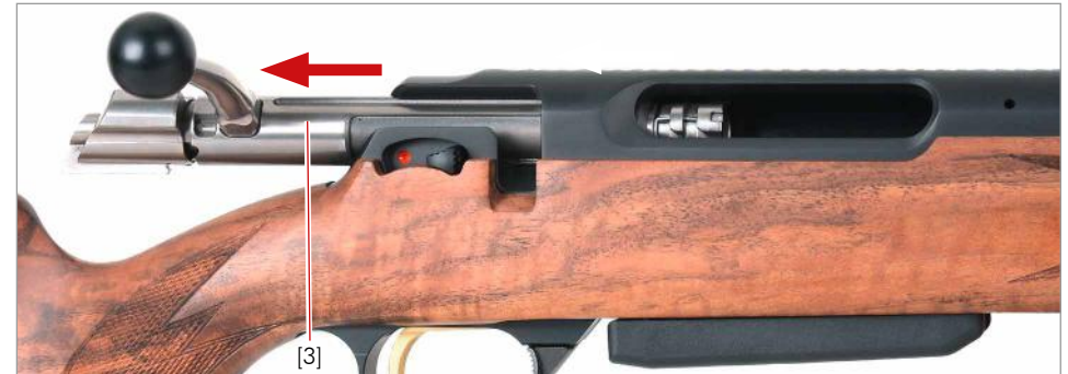
Fig. 11 Opening the breech
