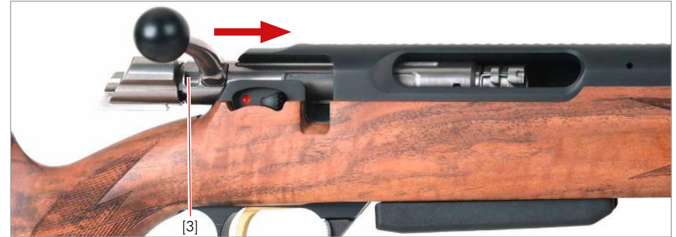
Fig.8 Closing the breech
