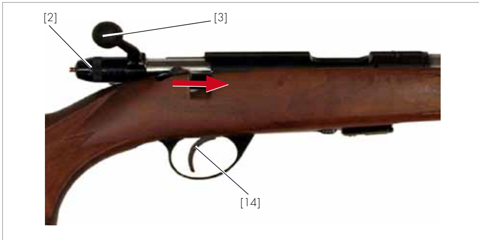
Fig.11 Closing the breech
