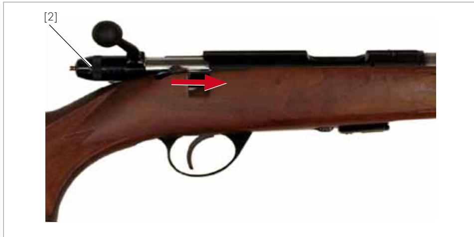
Fig. 13 Closing the breech
