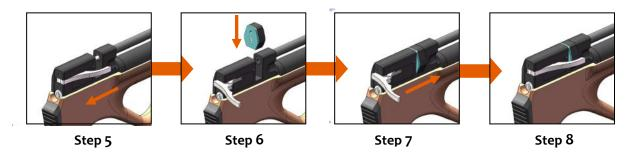
FIG 6 LOADING PROCEDURES
