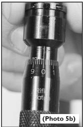
If this position does not align with the 0 mark on the Thimble **(Photo 6)** – do the following:
