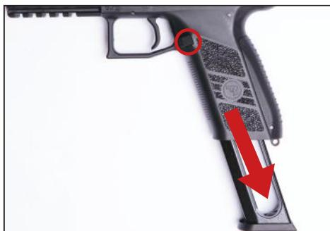
Push the Magazine release latch and pull out the magazine.
