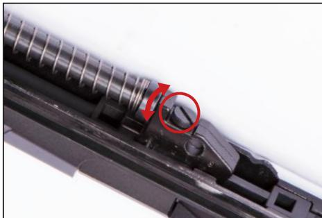
Gradually turn the lever from left to right and fire a round or two to see the effect. Continue to adjust until the BBs fly straight/horizontally. Perfect Hop-up is applied when the BBs fly straight.
