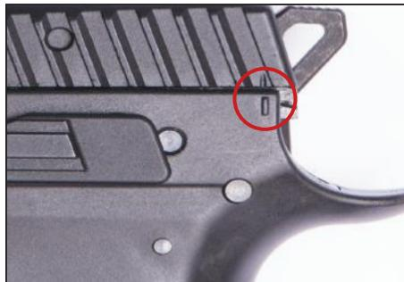
Remove the magazine. Pull back the slide and hold it over the first (the smallest) of the two grooves on the left side of the pistol.
