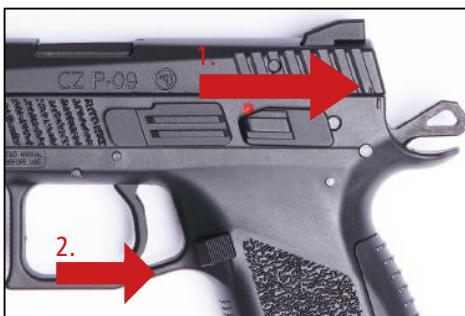
To fire the gun: 1. Pull back the slide. 2. Push the trigger when ready to fire.
