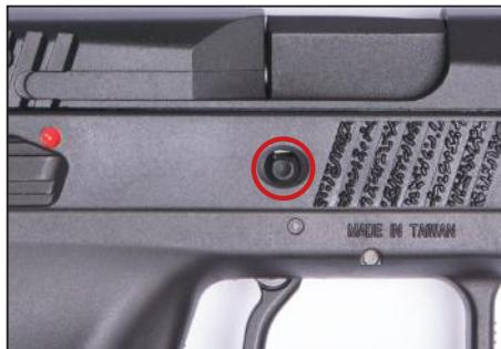
While holding the slide back over the small groove, press in the pin on the right side of the pistol. You can use a small screwdriver or pen to press in the pin and thereby remove the pin/slide stopper from the pistol.
