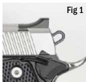
Fig 1 Fully down or "at rest" position (Fig 1). Hammer resting directly against the slide.
