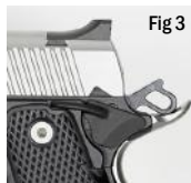
Fig 3 Fully Cocked Position (Fig 3). The hammer is fully rearward to the end of its travel. When there is a live round in the chamber and the safety is in the off position, the pistol is now ready to fire.
