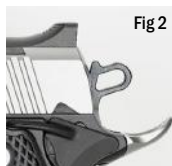
Fig 2 Half Cock Position (Fig 2). The hammer is between the fully down and fully cocked position (approximately 1/4" from fully down position). DO NOT CARRY YOUR BUL SAS II OR STORE IT WITH THE HAMMER IN THE HALF COCK POSITION.
