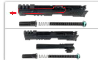
Remove the barrel.
