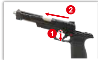
1. Push down the take-down lever. 2. Push the slide forward.
