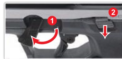
Rotate the take-down lever and press down the slide stop.
