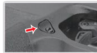
Turn the pistol to the other side and find the slotted drive screw on the magazine release button.
