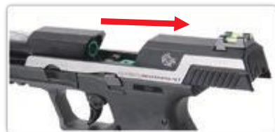
Pull the slide and push up the slide stop to lock back.
