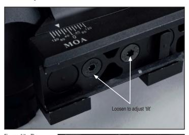
Figures 4/4a: The mount's 'tilt' screws are located under the clamp. Loosen both bolts, adjust the tilt angle and retighten. Use the vernier on the side of the mount base as a reference
