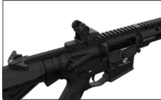
The bolt moving backwards pushes the striker backwards and re-cocks it. The locking spring with buffer housed in the rifle's buttstock ensures that the bolt closes again after the end of the rearward motion. In the process, a new cartridge is moved from the magazine and into the chamber. The rifle is re-cocked and ready to fire.
