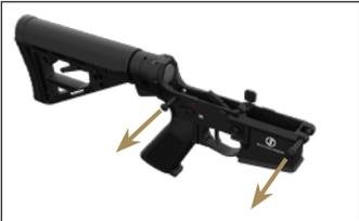
3. Place upper receiver onto lower receiver. First, push the front retaining pin all the way in, then tilt the upper downwards and slide in the rear retaining pin
