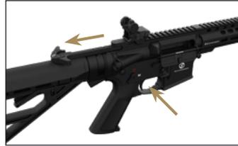
5. Slowly guide the trigger forward. The disconnecter will release the striker. This will make a “click” sound. Pulling the trigger will fall the striker
