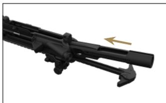
3. Push the charging handle with the bolt group simultaneously forward until it locks into the barrel extension
