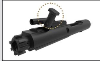
3. Guide the firing pin backwards from the bolt head carrier and remove downwards
