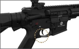
3. Set safety lever to position
