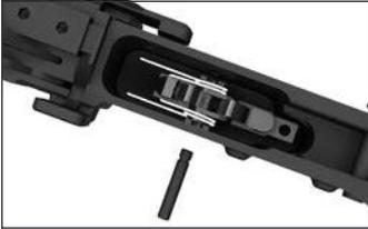
2. Align the hammer in the lower receiver. Make sure that the legs of the hammer spring point backwards and rest on the trigger pin. Push in the hammer pin with its notch on the right side through the hole of lower receiver and hammer
