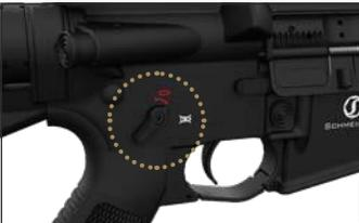
4. Hold the trigger down and cock the rifle using the charging handle at the same time; the disconnecter will hold the striker in the rearward position
