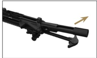
3. Pull back the charging handle up to the recess in the upper receiver and remove it upwards
