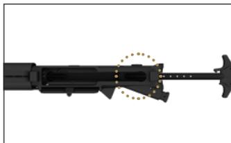
2. Insert bolt group into recess in the charging handle with the gas diverter facing downwards (make sure that the bolt head has been pulled all the way to the front so that the locking piece is in the maximum forward position)
