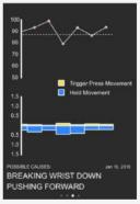
Trace view. This shows the detailed trace of the movement of the firearm. Blue is movement while holding on target. Yellow is movement during trigger press. Red shows the recoil of the firearm after the shot.
