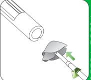
11. Dry rear of bolt carrier w/ loop & patch. Refer to Figure B (to the right) for how to insert patch into loop.
