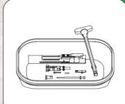
Place BCG parts in plastic container and soak with C4 Carbon Remover (C4).
