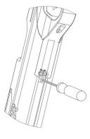
To change the batteries, simply remove the battery cover on the bottom of the housing by loosening the screw (fig.). Positioning of the batteries as shown on the bottom of the battery case.
